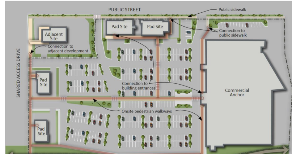
FIGURE 29: Required On-site Pedestrian Walkways
